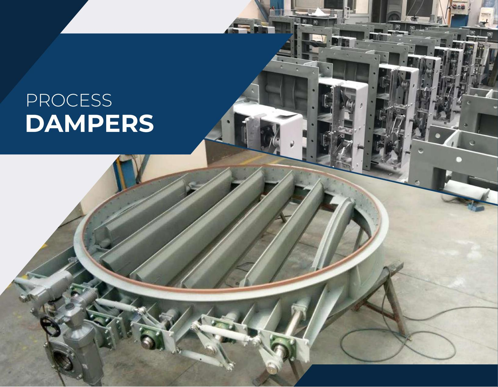
We provide reliable and cost-effective solutions for the design, manufacture and erection of many dampers such as butterfly, tight shut-off louvre, fully sealed multi louvre, tri lever and guillotine dampers. These dampers successfully control the gas flow from any process of power and many industrial applications. They are also used for component isolation for maintenance, emergency isolation or energy saving.
