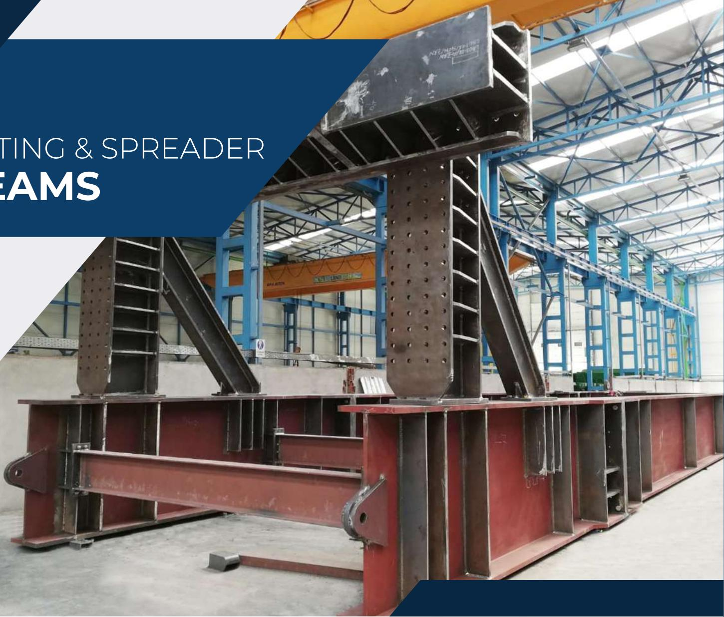
Besides our main products, we produce heavy lifting and spreader beams and uprighting frames for industrial services. These beams are designed and manufactured as per international standards, tested up to 700-ton loading with our special loading machine in our workshop. All beams are offered with CE certificates.
